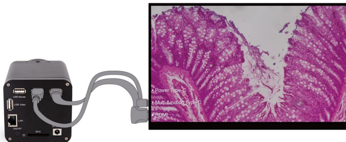
Figure 15 TAFDM411 Series Camera Connected to Touch Screen
